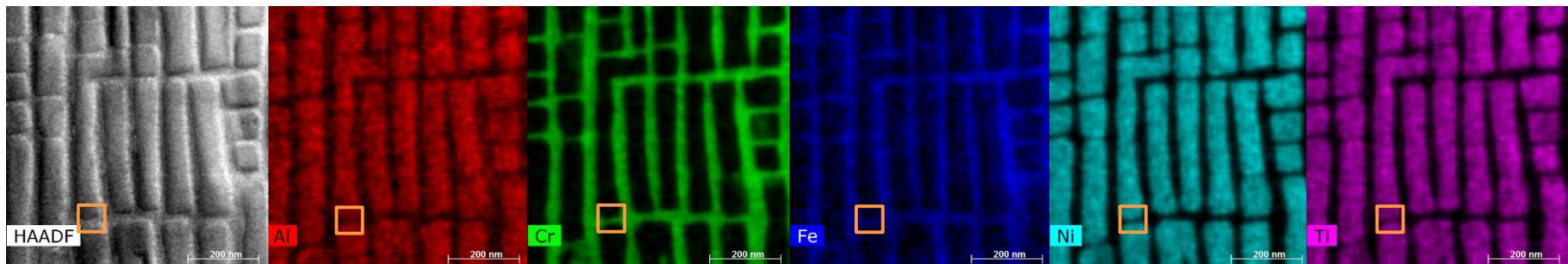
EDS-PCA gives quantified composition in separate phases
