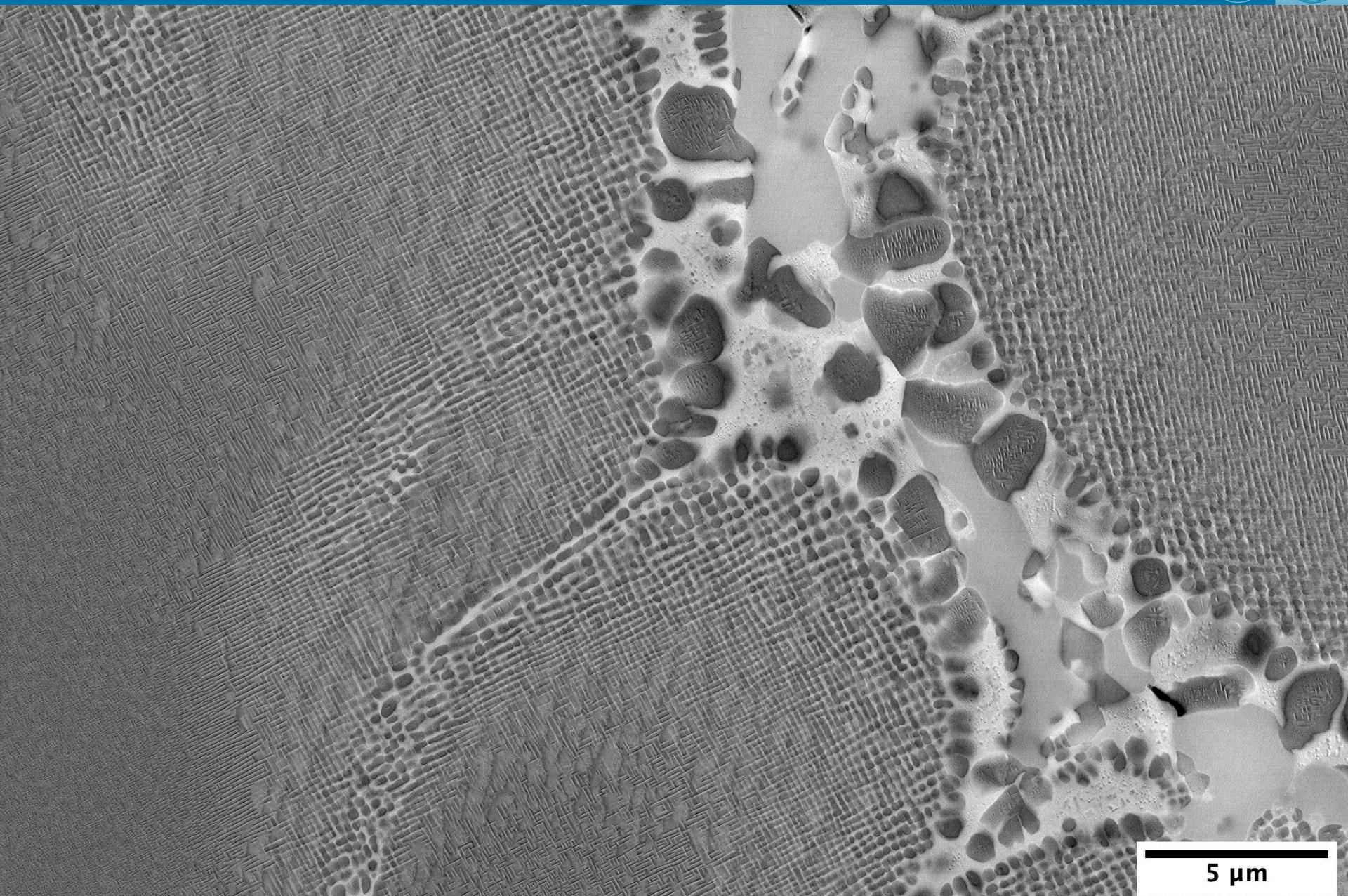
SEM Microstructures – C11 –  $\text{Al}_{25}\text{Cr}_{15}\text{Fe}_{30}\text{Ni}_{20}\text{Ti}_{10}$
