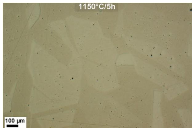
Fig. 9. Optical micrograph of Al<sub>8</sub>Co<sub>17</sub>Cr<sub>17</sub>Cu<sub>8</sub>Fe<sub>17</sub>Ni<sub>33</sub> heat treated at 1150°C/5 h alloy showing annealing twins.
