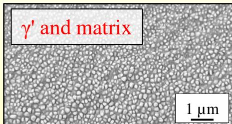
Finely distributed  $\gamma'$ -particles in a fcc-matrix
