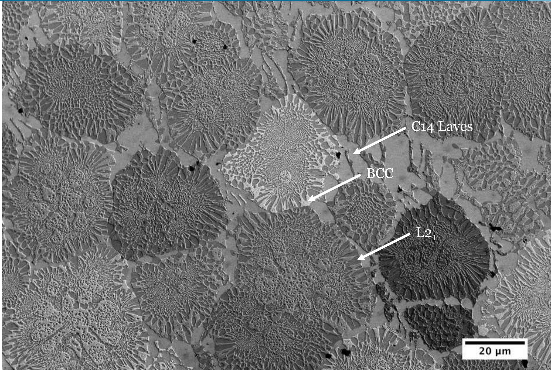
SEM Microstructures – B<sub>12</sub> – Al<sub>20</sub>Cr<sub>10</sub>Fe<sub>35</sub>Ni<sub>20</sub>Ti<sub>15</sub>
