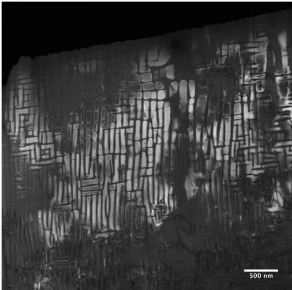
Two beam diffraction condition with  $<110>$
