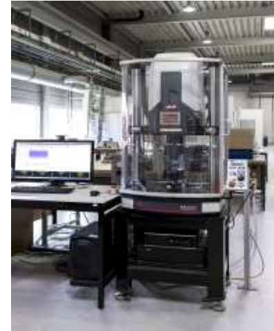
MTS Acumen™ Electrodynamic Test Systems 100 Hz, \pm 3 kN
